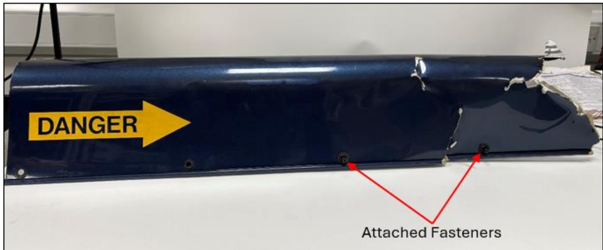
Photo No. 3: Left-hand side view of damaged fairing
