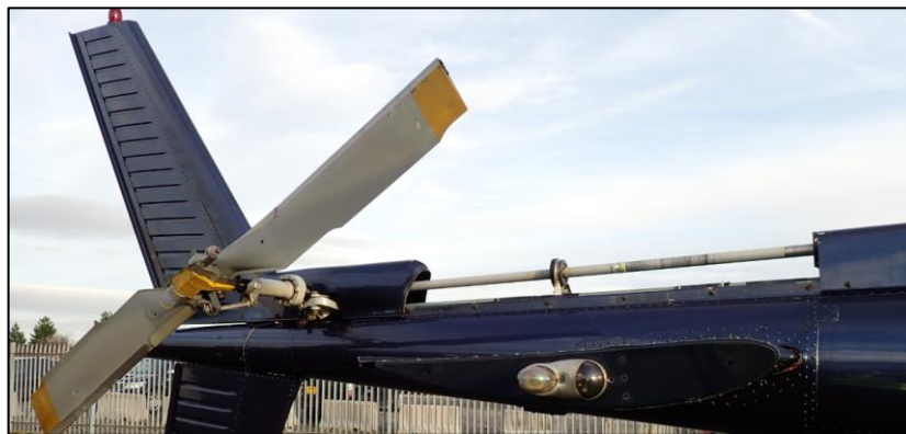
Photo No. 1: Exposed section of tail rotor driveshaft
