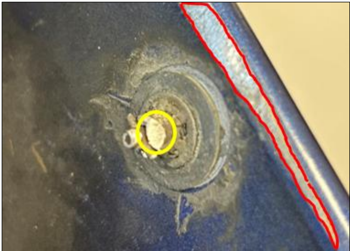
Photo No. 4: Damage to fastener and lip of fairing
