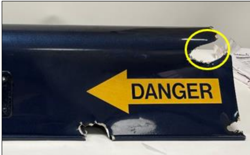
Photo No. 5: Damage to fairing
