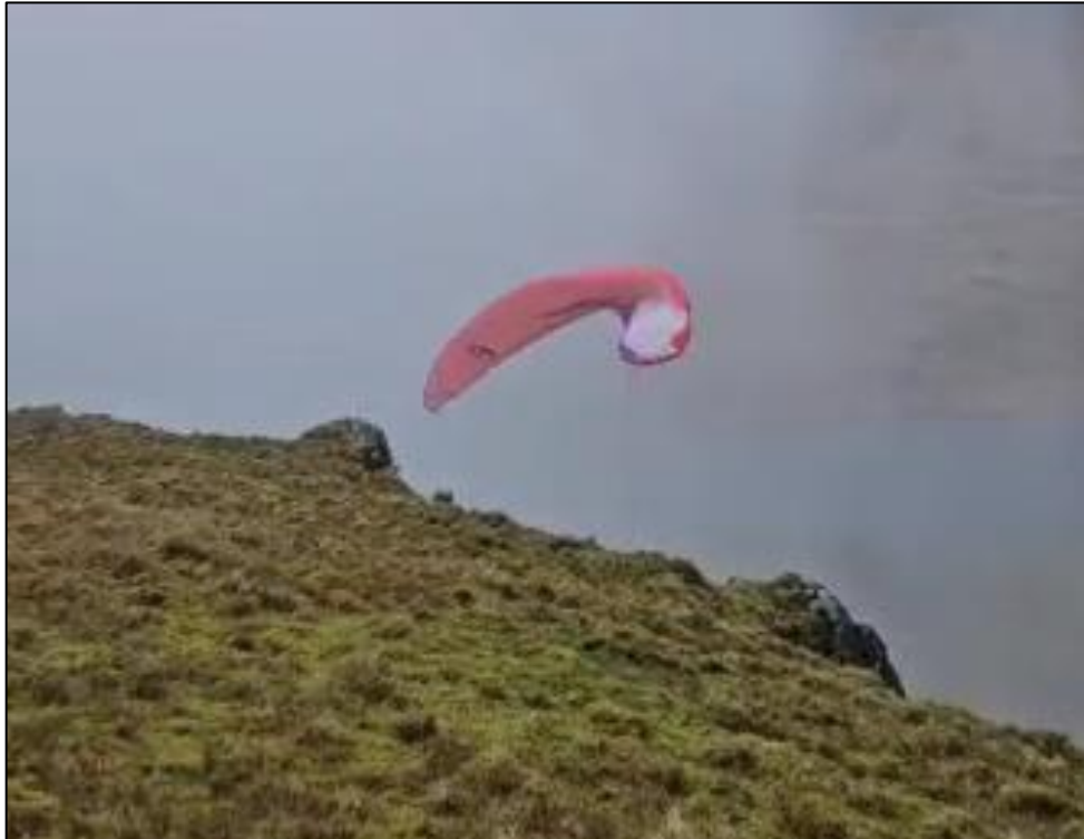
Photo No. 1: Asymmetric canopy collapse on the right-hand side (with low cloud obscuring the valley below)
