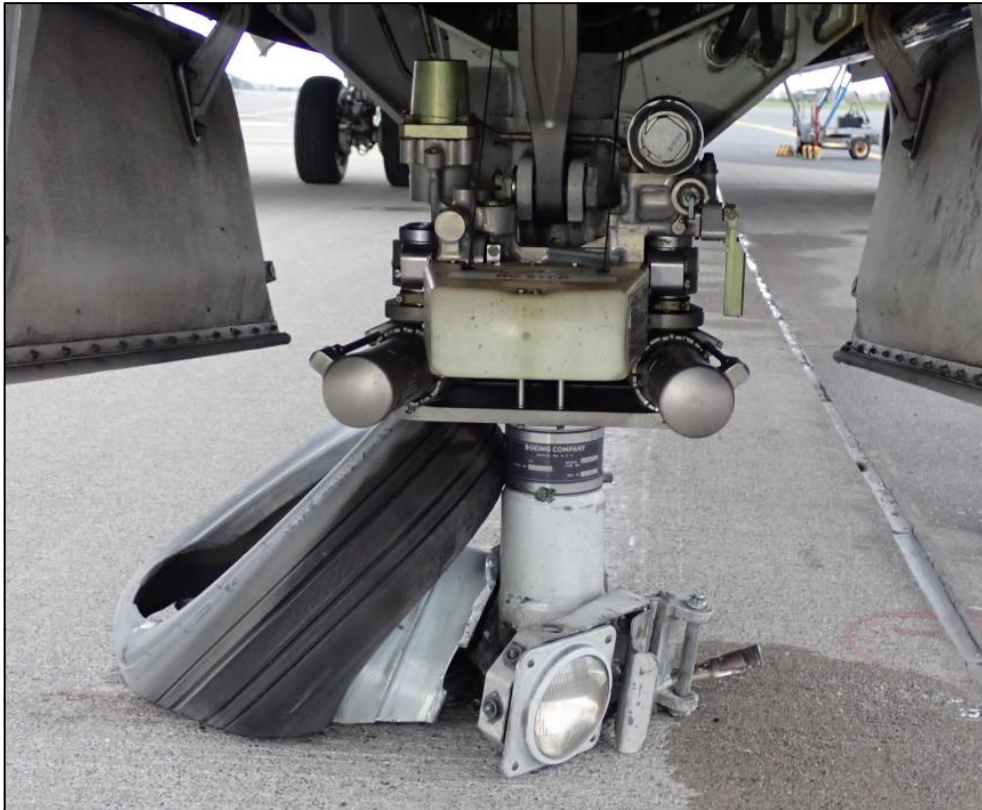
Photo No. 1: NLG assembly as the aircraft came to rest
