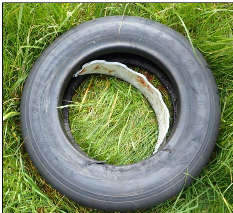
Photo No. 3: Left-hand tyre and section of wheel hub
