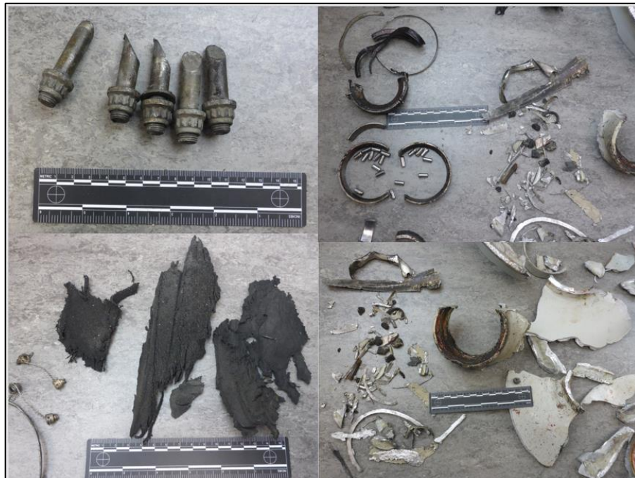
Figure No. 2: Sample of the fragments recovered from the runway
