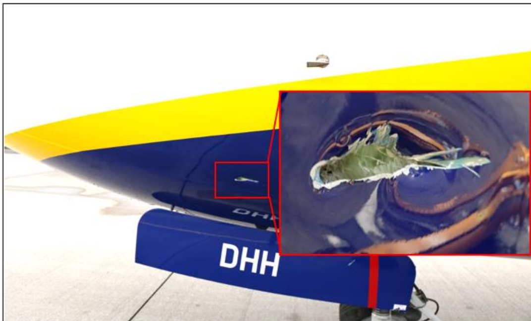
Photo No. 5: Punctured fuselage skin on left side of aircraft
