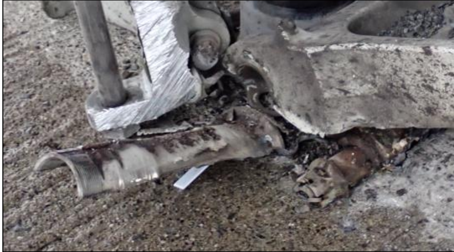
Photo No. 4: Ground down axle
