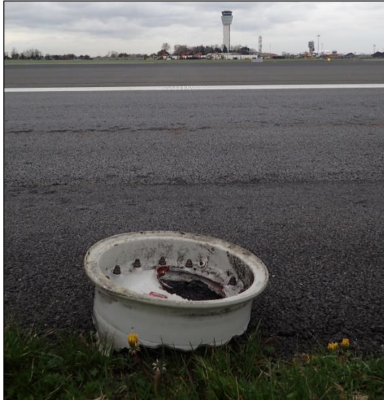
Photo No. 2: Portion of left-hand wheel at runway edge
