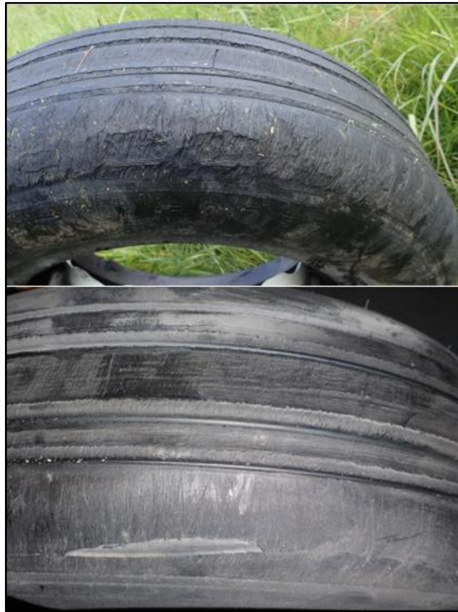
Figure No. 3: Examples of the abrasion marks on the left (top) and right (bottom) tyres
