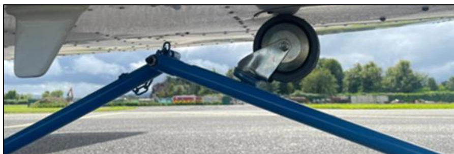
Photo No. 2: Towbar's wheel in contact with inspection panel ( image provided by AFRS )
