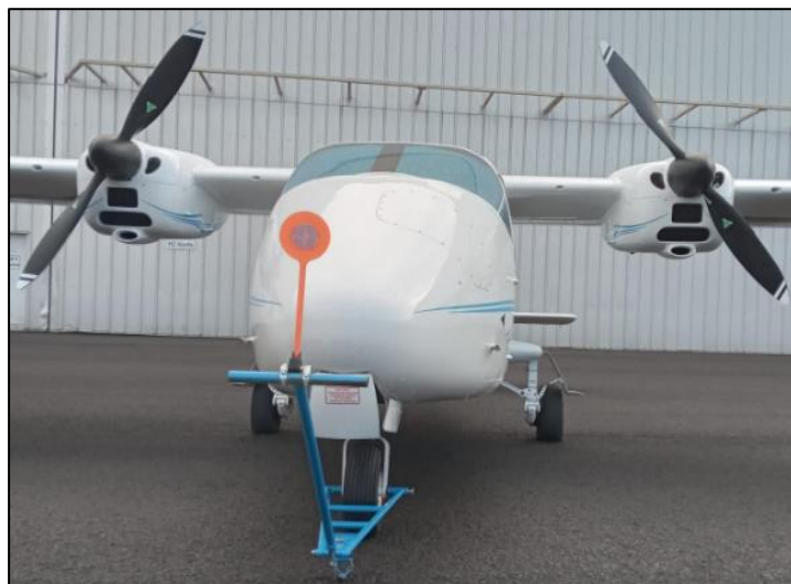
Photo No. 5: Modification to towbar
