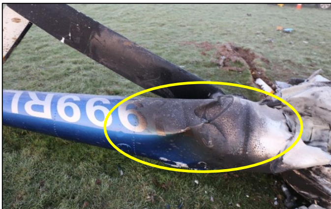
Photo No. 7: Fire damage and crumpling to tailcone (highlighted) (Photo taken on the morning after the accident)
