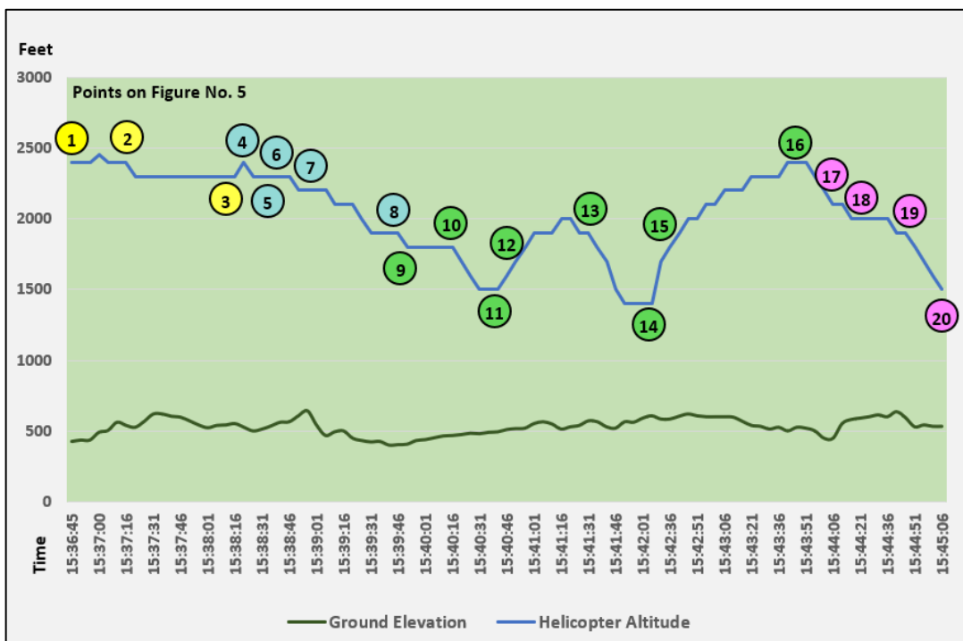
Figure No. 6: Altitude profile as indicated by ARTAS data and ground elevation (Helicopter altitude corrected for the air pressure on the day)
