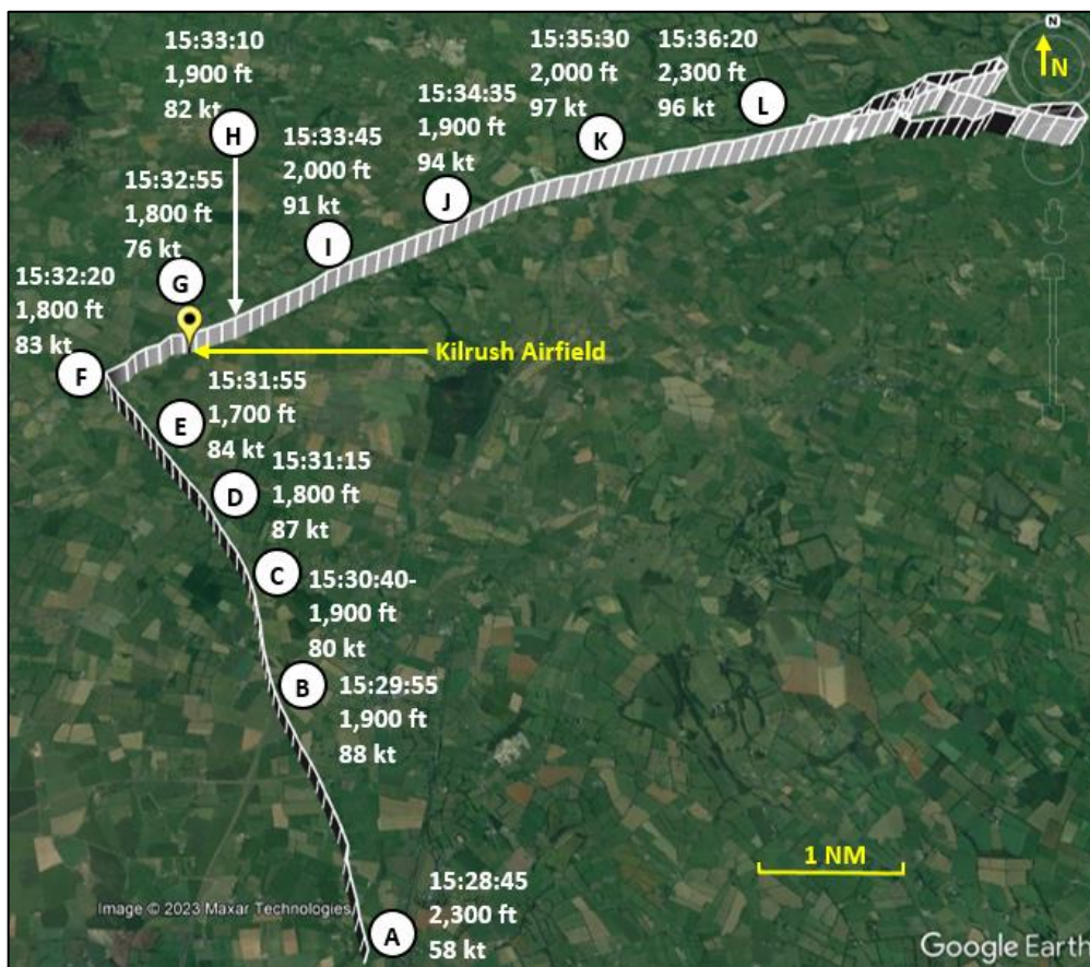
Figure No. 4: Flight path, with time, altitude (corrected for the air pressure on the day), and ground speed as indicated by ARTAS data ( Note: The terrain image is historic and does not represent the meteorological conditions prevailing on the day of the accident)
