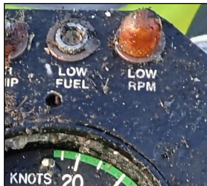
Photo No. 13: Instrument panel with warning light assemblies
