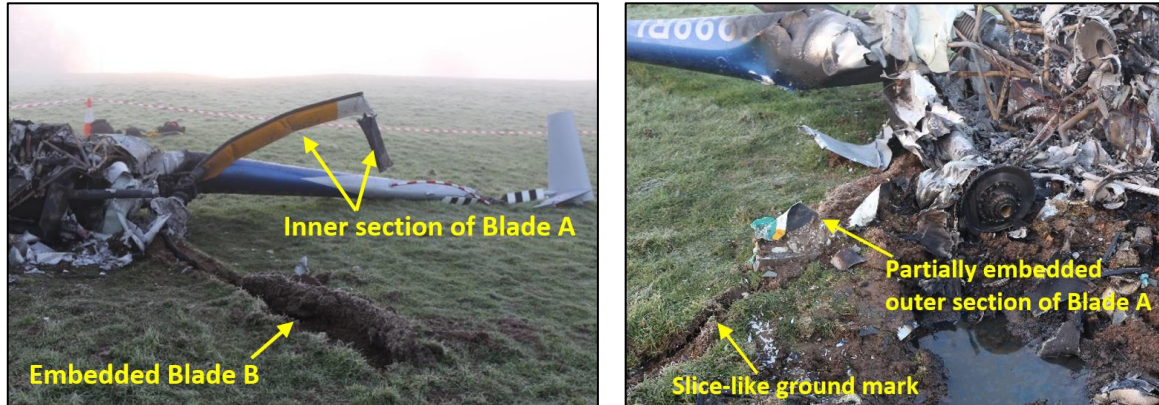
Photo No. 5 (left) and Photo No.6 (right): Damage to main rotor blades and surface of field (Photos taken on the morning after the accident)
