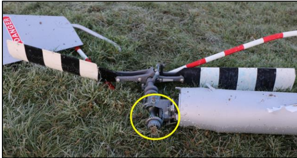
Photo No. 9: Broken tail rotor gearbox (circled) (Photo taken on the morning after the accident)
