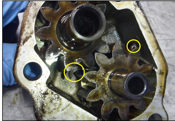
Photo No. 16: Metallic chips in the engine oil pump (circled)
