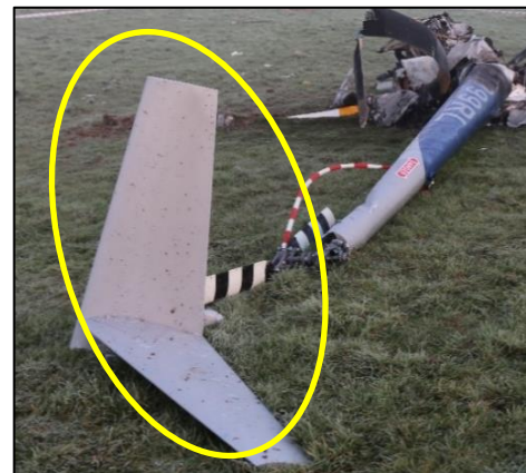
Photo No. 8: Separated empennage (highlighted) (Photo taken on the morning after the accident)
