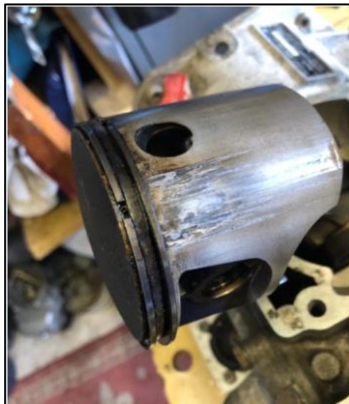
Photo No. 2: Damaged forward piston
