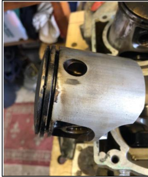
Photo No. 3: Rear piston exhibiting loss of clearance damage
