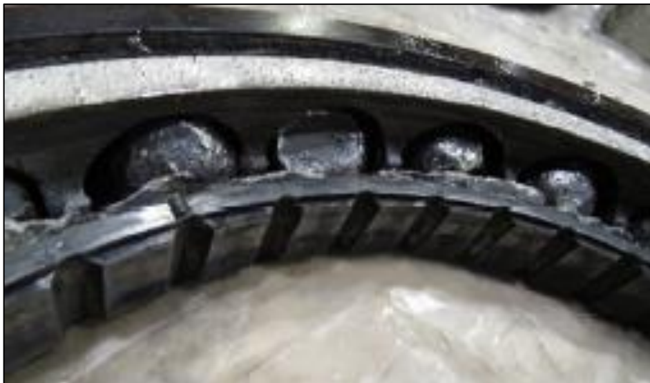
Photo No. 2: Engine No. 1 Bearing post Occurrence ( Courtesy of Engine Manufacturer )
