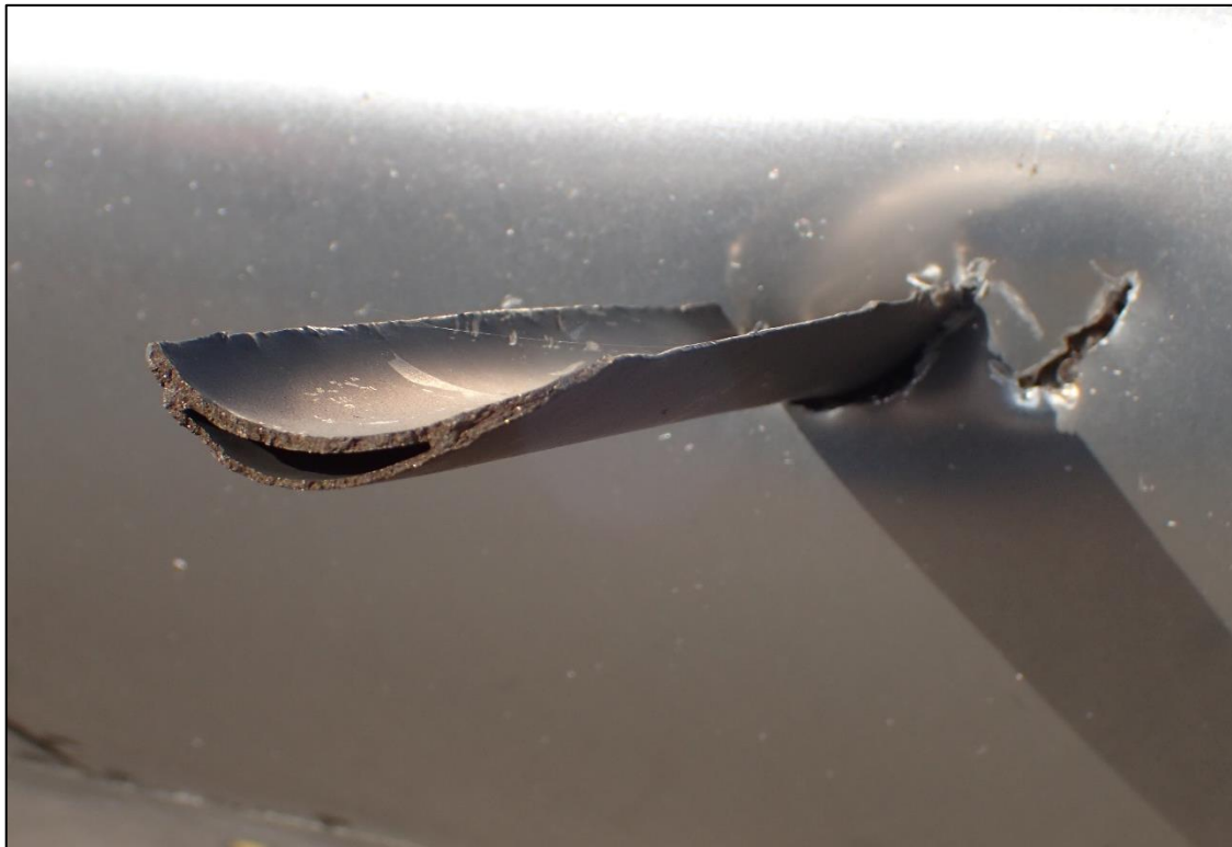
Photo No. 1: Turbine blade impact with horizontal stabiliser
