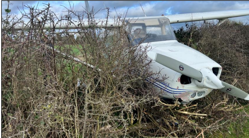
Photo No. 2: Final position of EI-GWU showing aircraft damage
