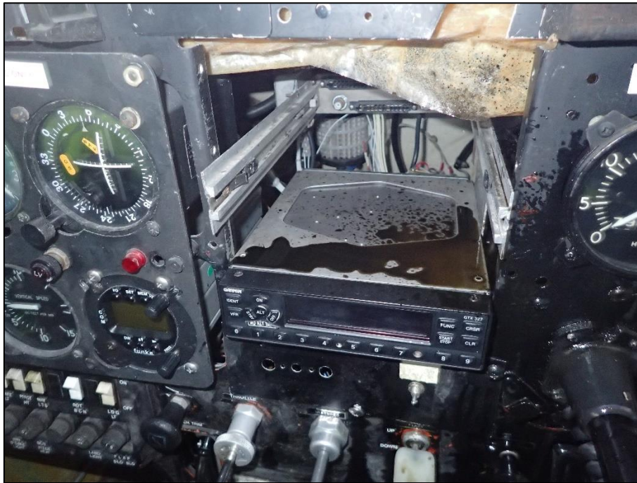
Photo No. 3: Open instrument panel with oil pooled on transponder unit
