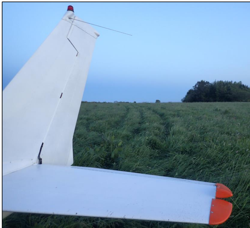
Photo No. 2: Curved ground track made by the aircraft wheels
