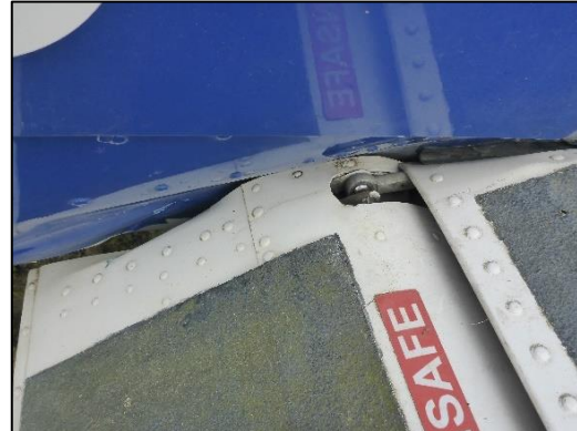
Photo No. 5: Damage to flap and fuselage
