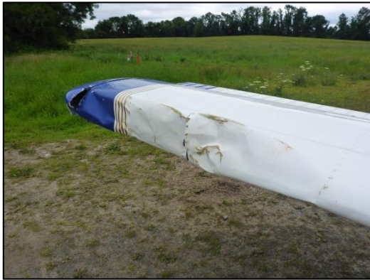
Photo No. 2: Damage to right wing
