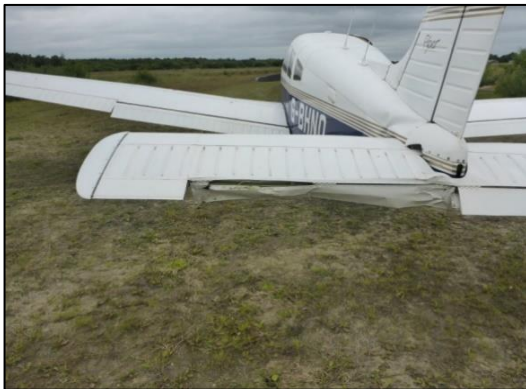
Photo No. 4: Damage to left anti-servo tab
