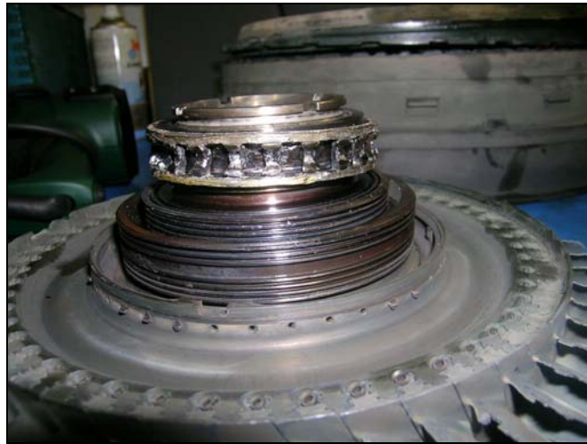
Above, the deformed and fused No.6 bearing
