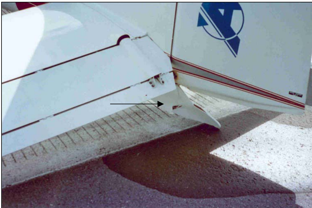
Arrow indicating damage to ventral fin assembly
