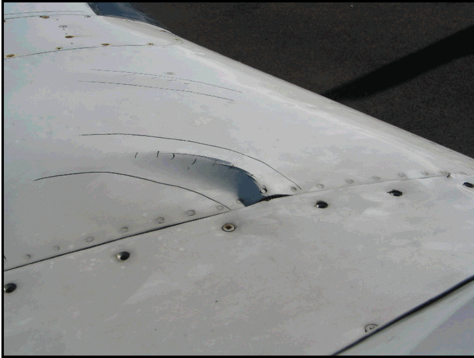
Photo 1 Buckling on port wing at outer wing panel joint
