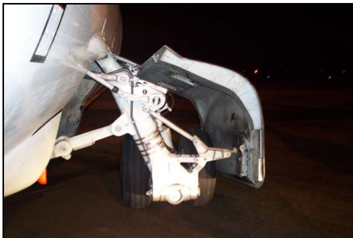
Photo No. 3: General view of the LH undercarriage and door.
