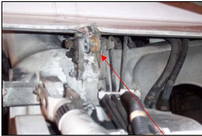
Photo No. 2: The corresponding half fixed to the undercarriage strut showing the corrosion on the bearing housing.
