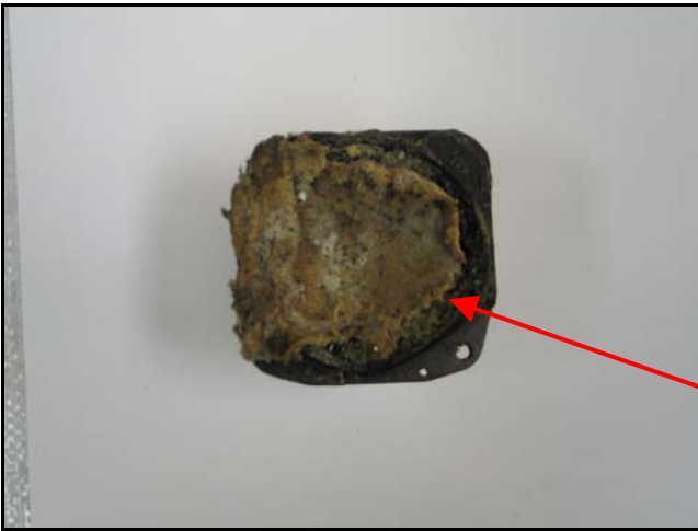
Altimeter No. 1 with face covered
