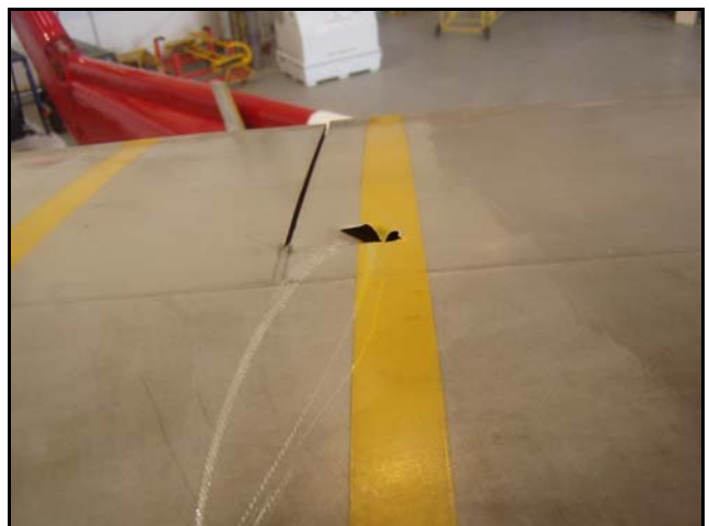
Photograph No. 3 - Damage to Black Blade
