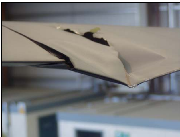
Photograph No. 2 - Damage to White Blade
