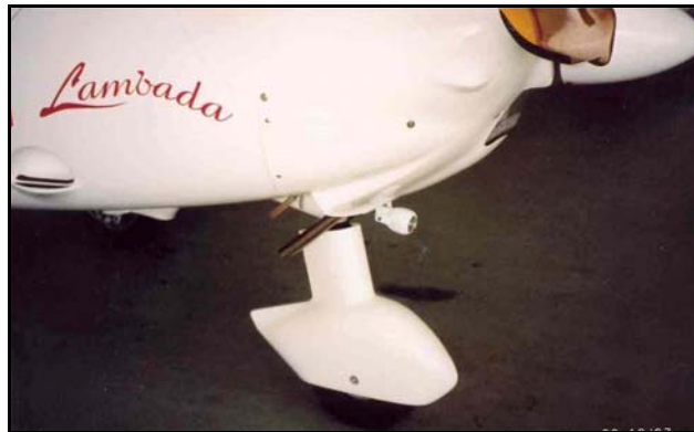
A serviceable nose wheel strut in a similar aircraft
