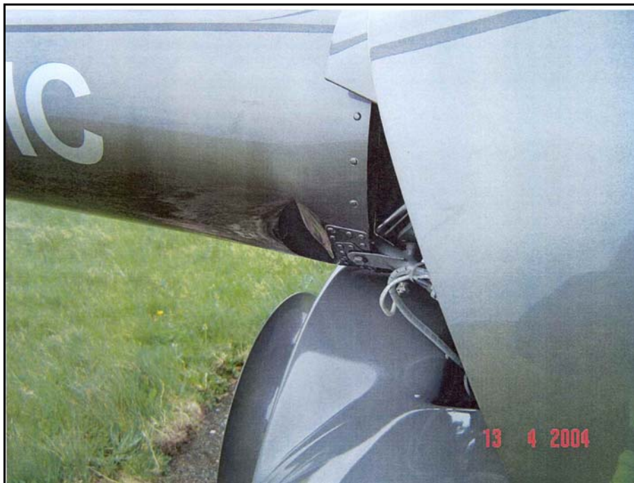
Buckling of the skin caused by compressive forces on the tailcone. (i.e. the skin is pushed in)
