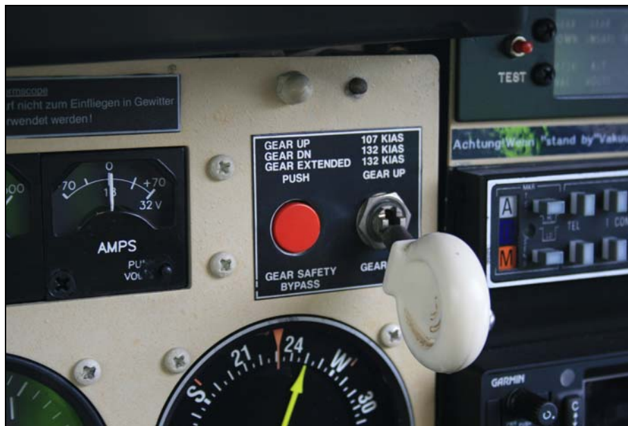
Photo No. 1: Landing Gear selector switch and Gear Safety Bypass switch
