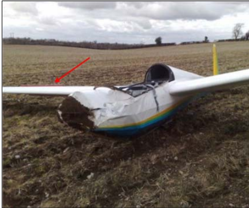
Photo No. 1: Damage to EI-GLD and part deployment of airbrake above and below wing (red arrow)
