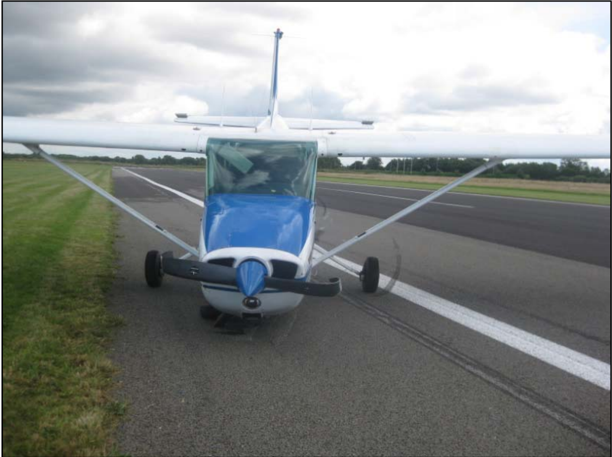
Photo No. 1: Nose wheel and propeller damage
