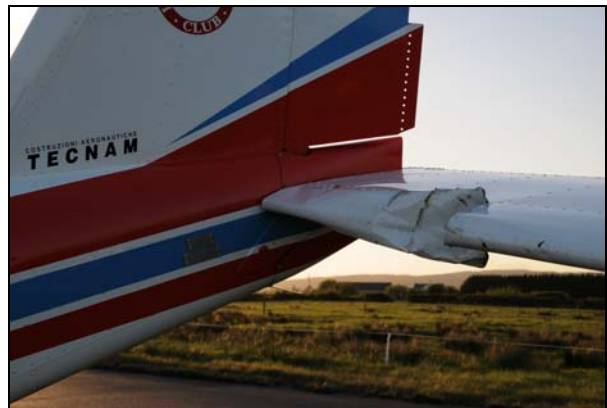
Photo No. 3: Damage to left stabilator
