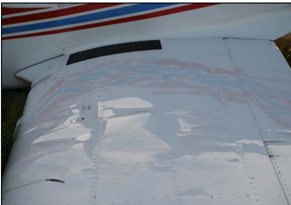
Photo No. 2: Damage to left wing
