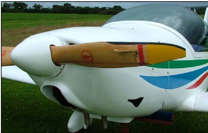
Photo No. 1: Propeller damage
