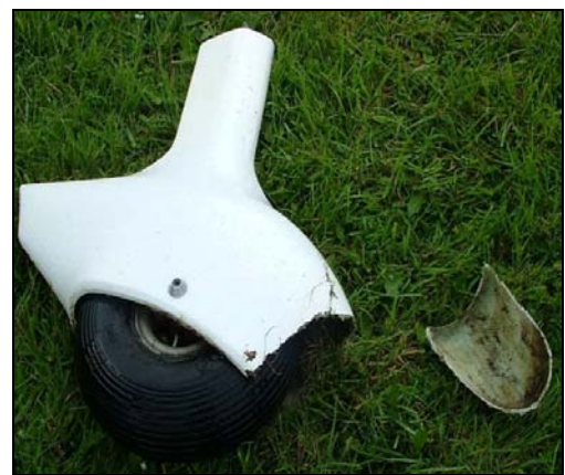
Photo No. 2: Severed nose wheel strut
