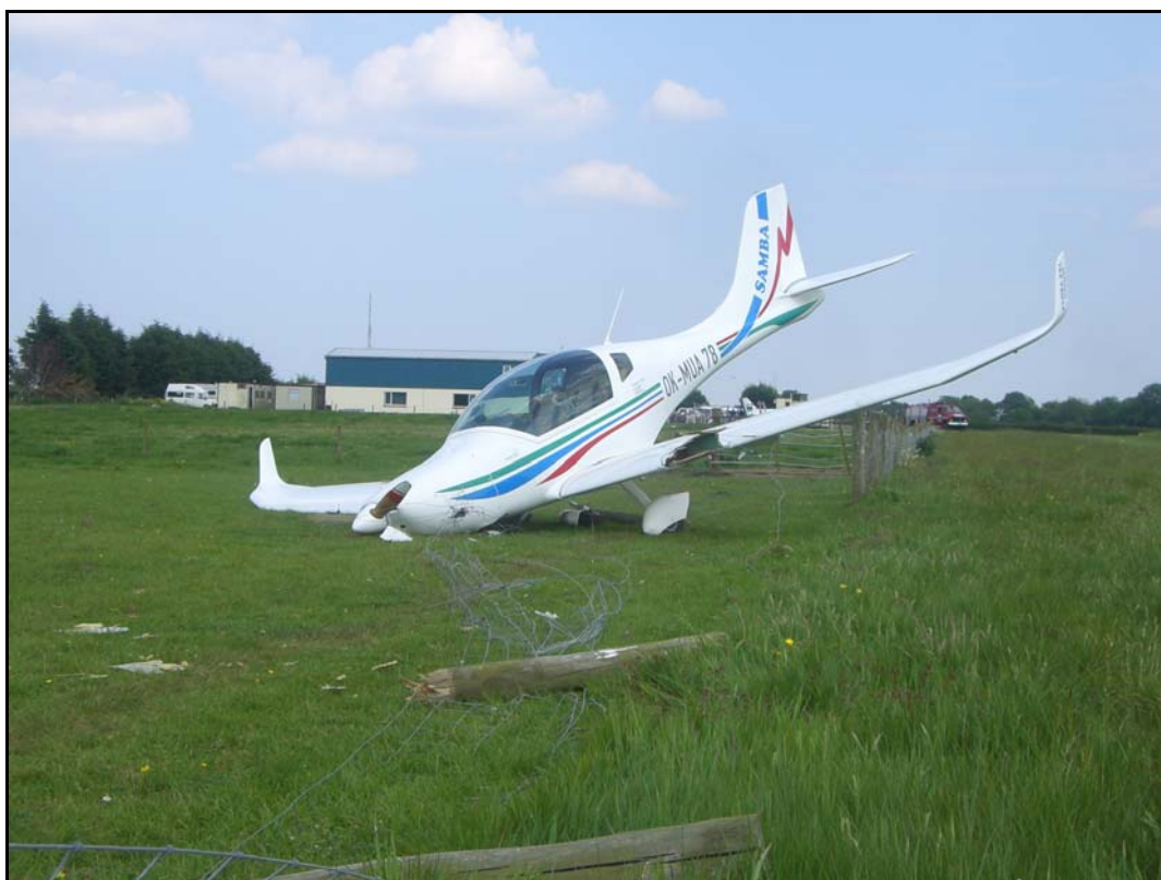
Photo No. 1: Impacted airfield boundary wire fence and broken posts.
