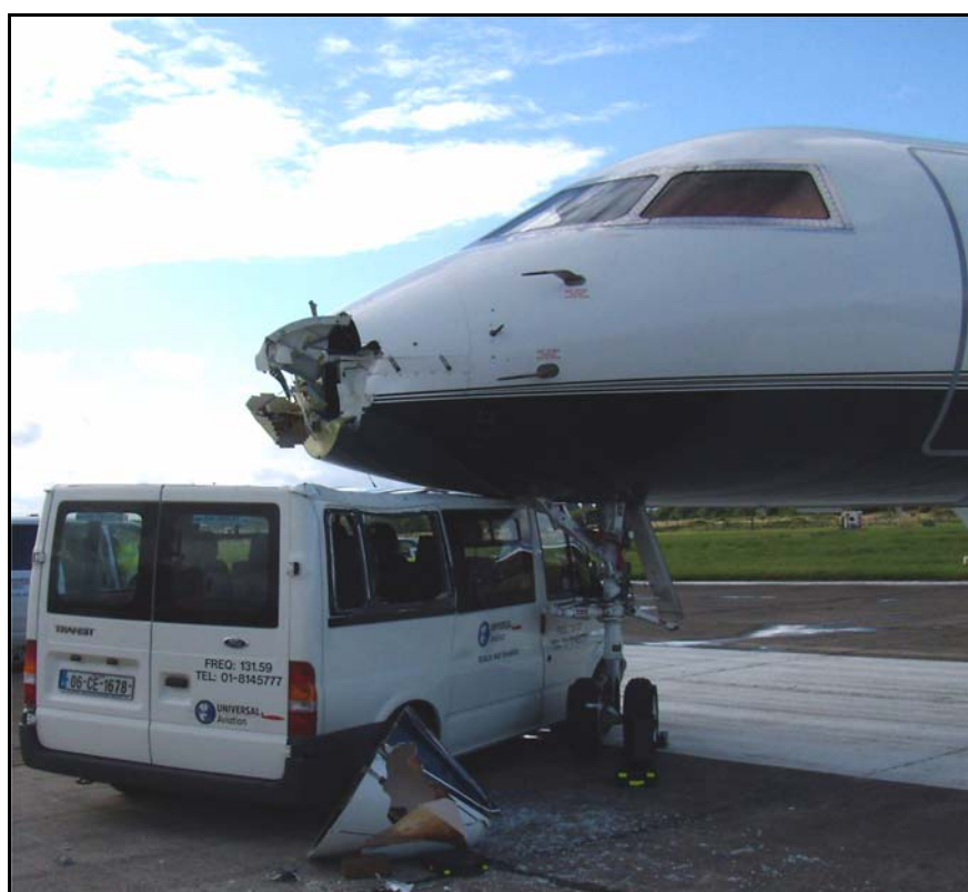
Photo No. 1: Damage to N20EG and Marshaller's van
