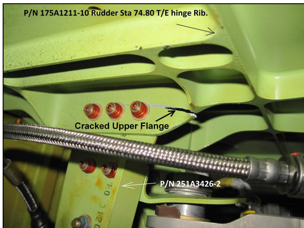
Photo No. 1: Damage to Standby PCU Support Bracket
