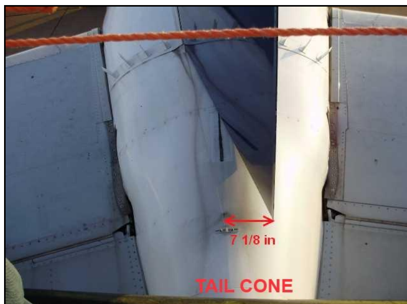
Photo No. 4: Rudder Trailing Edge Offset from Neutral
