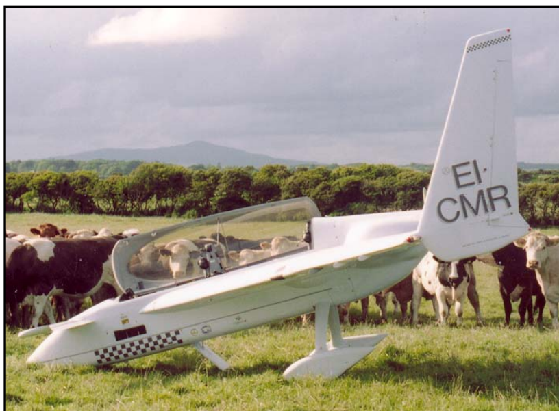
The aircraft, with its nose undercarriage retracted, following its forced landing in a field at Bunmahon, Co. Waterford.
