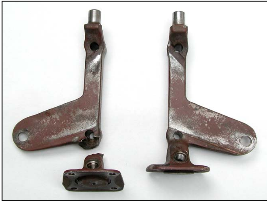
The 7.5 inch long fractured LH Saddle Assembly P/N 1241423-1 (Forging P/N 1241423-497) and cracked RH Saddle Assembly P/N 1241423-2 (Forging P/N 1241423-498).
