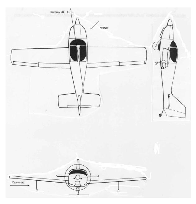
Sketch of the Europa Classic monowheel homebuild aircraft. Cables from the rudder pedals are linked directly to the tailwheel designed to provide positive steering on the ground. The outriggers with small wheels rotate to the horizontal when the flaps are retracted.
