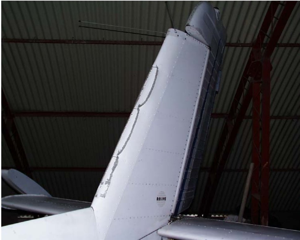
Photo No 1. Cable impact damage to leading edge cowling of vertical tail fin
